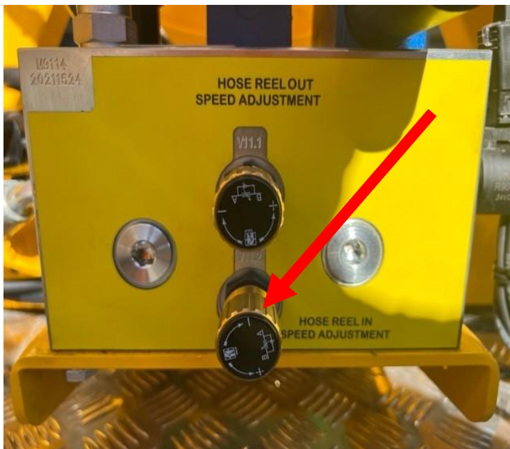
4. Main Hose Reel Speed Control – Hose IN - Bottom Dial
